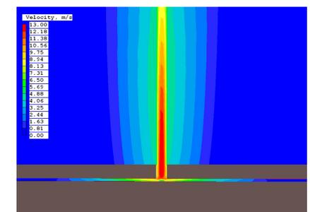
A steady-state case showing the gas velocity beneath the ice layer. Velocities in excess of 10 m/s are evident in the cavity.
