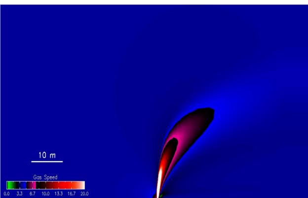
Model result showing the gas speed in a jet in the presence of a 4 m/s wind from the left. Velocities > 20 m/s are shown in white.
