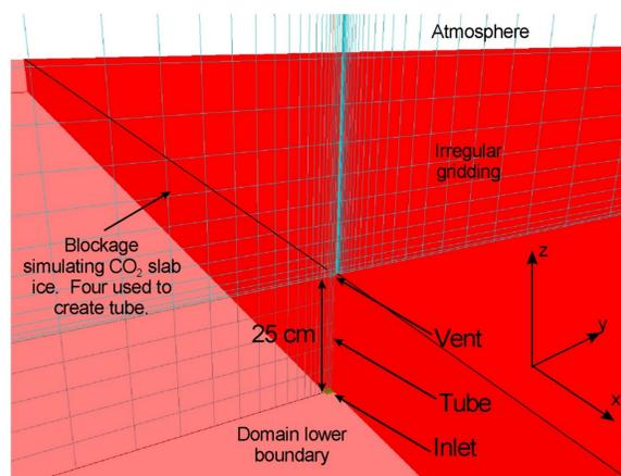
The set-up of the explosive model using an irregular Cartesian grid.
