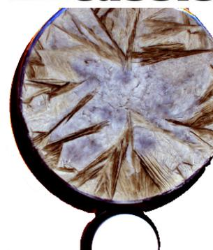
The colour picture on the left shows a sample prepared by freezing a preparation of wet smectite clay. The sample was then inserted into the SCITEAS simulation chamber and hyperspectral images regularly acquired as the ice sublimated in the low temperature / low pressure environment.
