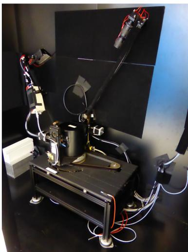
The PHIRE-2 instrument is a highly accurate and fully automated radio-goniometer that is operated at -30°C in a cold room to acquire measurements with icy samples [2]. It is used to measure the bidirectional reflectance with a high accuracy over wide ranges of incidence, emission and phase angles. Reflectance values were measured inside six discrete bandpasses between 400 and 1100nm.
