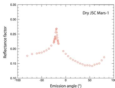
Recent improvements on the PHIRE-2 instrument now allow us to acquire measurements at low phase angle (down to 0°) and thus study in detail the opposition peak.
