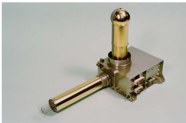
Figure 23: Picture of the ROSINA COPS-FS. The nude gauge is pointing to the left and the ram gauge is mounted on the top of the electronic housing. Connectors (with connector-savers) to the DPU are fitted into the right panel of the electronic box.
