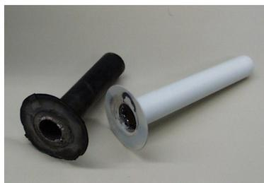
Figure 11: Crucible and hat for furnace
