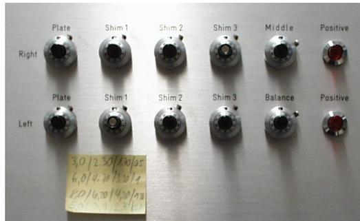
Figure 4: Knobs to adjust electrostatic values of Wien filter
